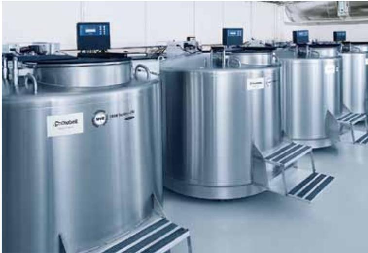
*Cryogenic freezing with nitrogen: Biomaterial can be stored without damage in cryogenic storage banks and tanks until it is needed (above). All cell activity stops when samples are submerged in liquid nitrogen at minus 196 degrees Celsius (right). Scientists can thaw the biomaterial decades later and use it for medical research (left).*
