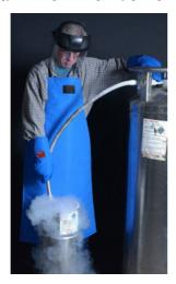
The face protection offered by LABOplus is made of clear, unbreakable polycarbonate. Compared to safety glasses its use is preferable, because it prevents steaming up and provides protection from splashes and vapors for eyes, face and neck.
